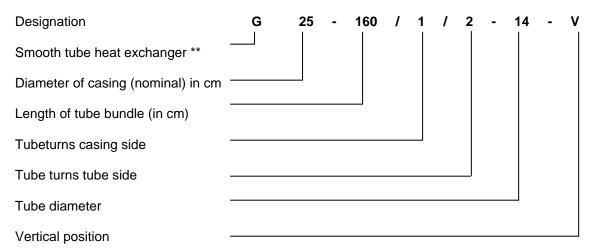
\*\* **GK**: Tube bundle condenser **GA**: Exhaust gas heat exchanger **GV**: Tube bundle evaporator **GS**: Safety heat exchanger
